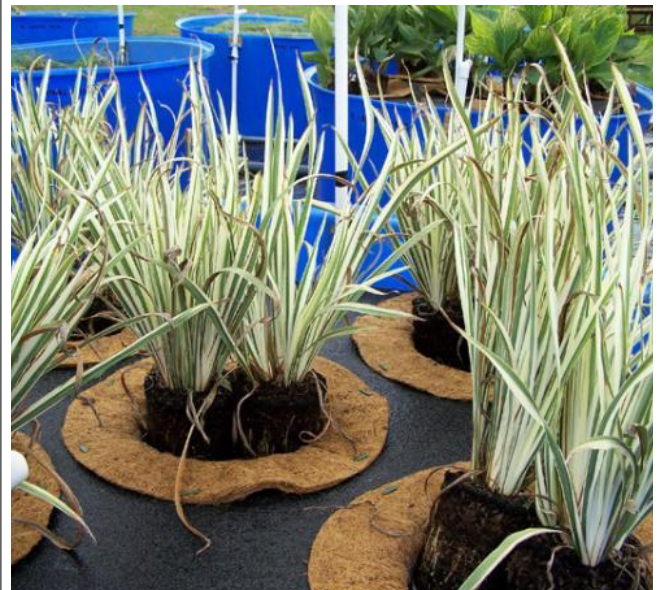
Plants can filter pollutants out of wastewater so the water can be reused. During S-1032 trials, iris plants (shown above), Bermudagrass, and wild millet grew successfully on floating mats in a swine wastewater lagoon. In addition to removing excess nutrients from wastewater, the growing vegetation can be harvested, composted, and used as a soil fertilizer, or transplanted as sod. Photo by Rob Hubbard, USDA-ARS.
